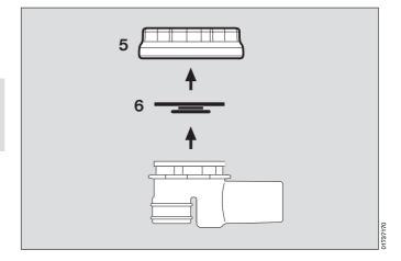
The rubber disc in the housing must not be removed, damaged or bent, otherwise the valve will not work properly and endanger the patient.
