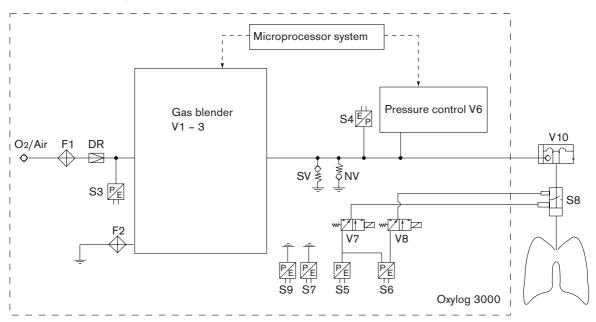
The variable pneumatic actuators in the Oxylog 3000 are controlled by the microprocessor system via digitized electrical test signals.
