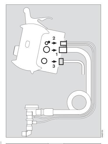
When disconnecting the ventilation hose, always grip the sleeve and not the corrugations!
